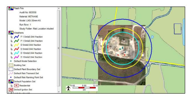
Figure C3- Flash fire of LNG metering 30 mm hole size
