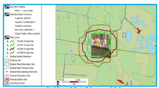
Figure 11. BNOCL LNG PLANT Outdoor LSIR Contours
