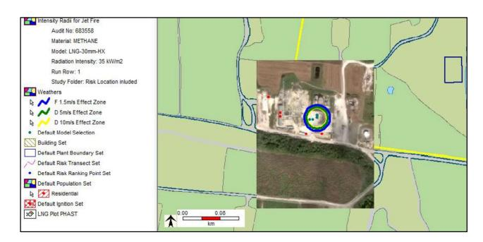
Figure C5- Jet fire radiation of LNG Vaporizer 30 mm hole size
