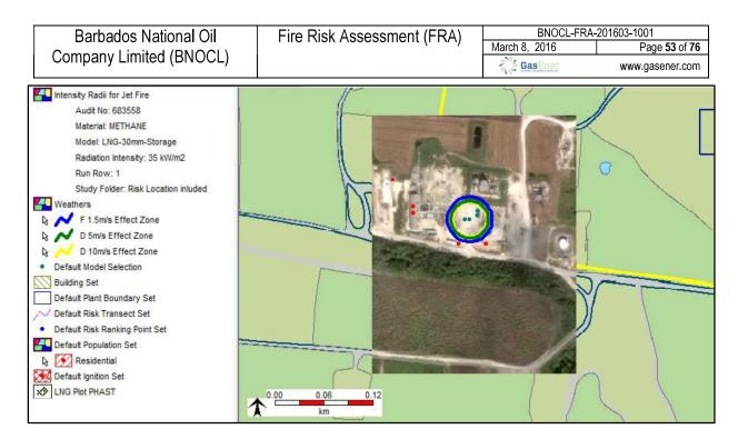
Figure C4- Jet fire radiation of LNG storage 30 mm hole size
