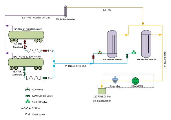
Figure 3. LNG plant schematic Process Flow Diagram (PFD)
