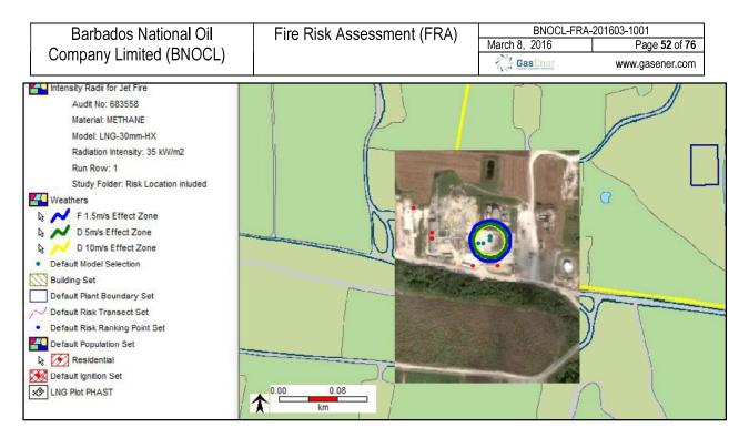
Figure C2- Flash fire of LNG Vaporizer 30 mm hole size
