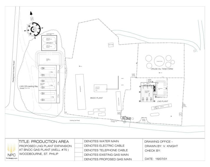
FIGURE 2-9 LNG PLANT LOCATION AND DISTRIBUTION OF ISO-CONTAINERS AND LNG STORAGE TANKS – DESIGN OPTION 3
