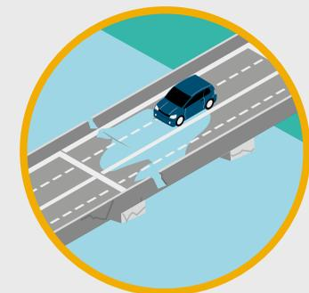
3 Erosion on margins and supports
